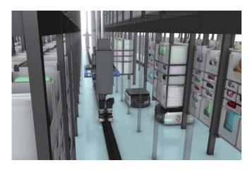
High capacity loading and unloading through combination of high speed cranes and AGV
